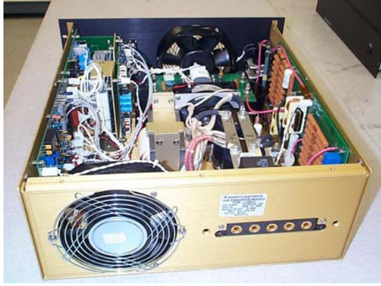
Figure 6. Photograph showing the converter.
