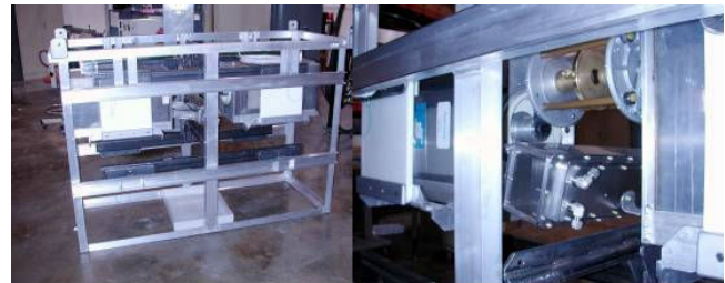
Figure 1. Capacitors, switch, and load in test stand.
