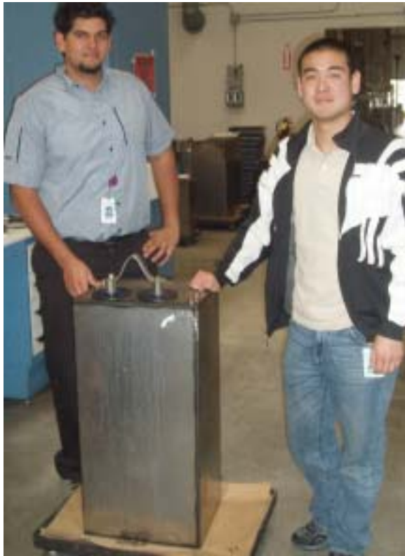
Figure 2- First Quarter-MegaJoule Capacitor
