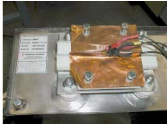
Figure 2. Impedance measurement made using a low inductance fixture on the DC link capacitor.
