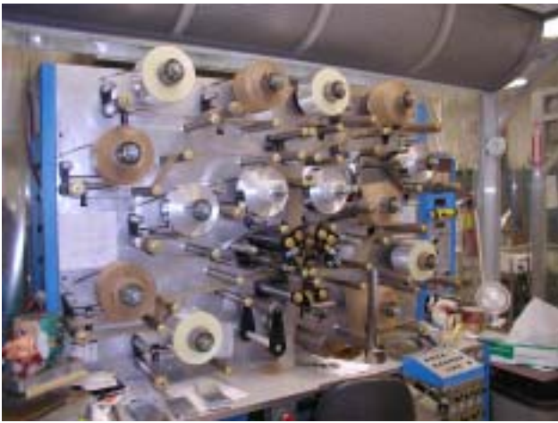
Figure 7. Winding machine for fabrication of capacitors.
