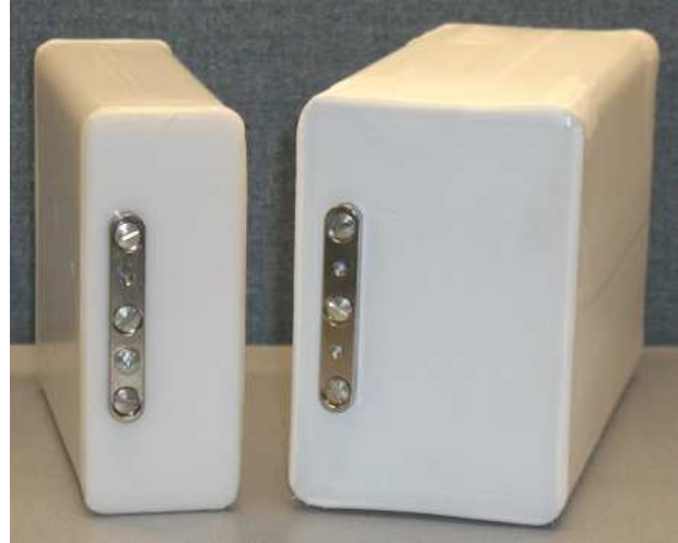
Figure 5. Examples of 100 kV capacitors for LTDs.
