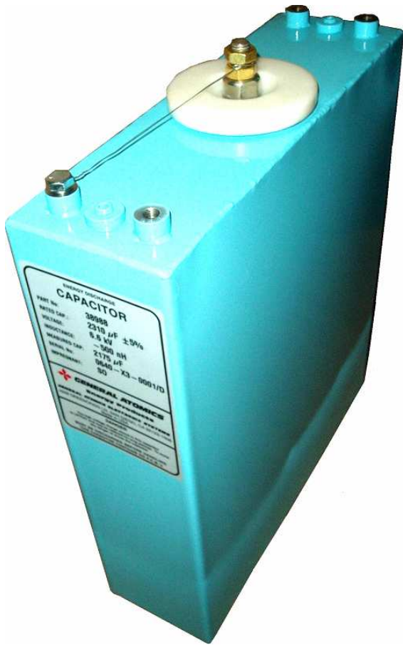
Figure 2. A 3.0 J/cc, 50-kJ capacitor.
